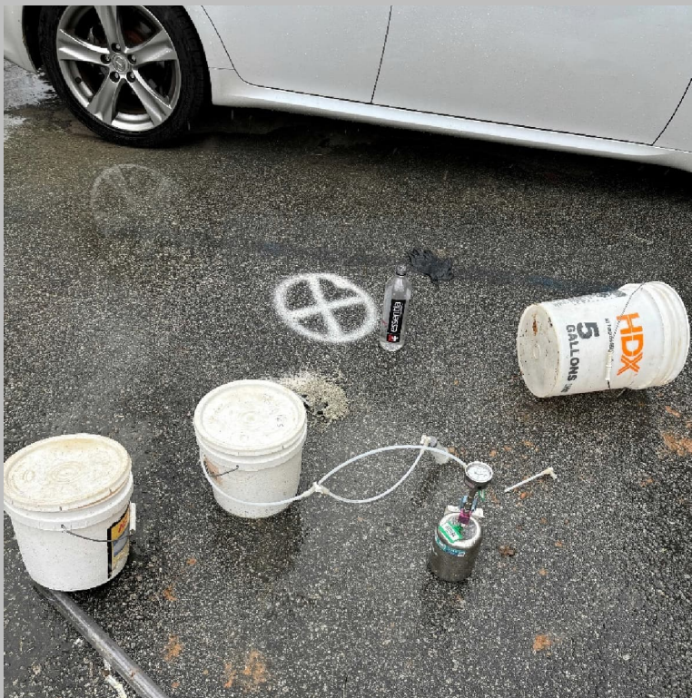
Photograph of soil vapor sampling for SG-1.
