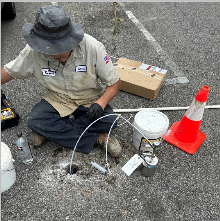
Photograph of soil vapor sampling for SG-3.
