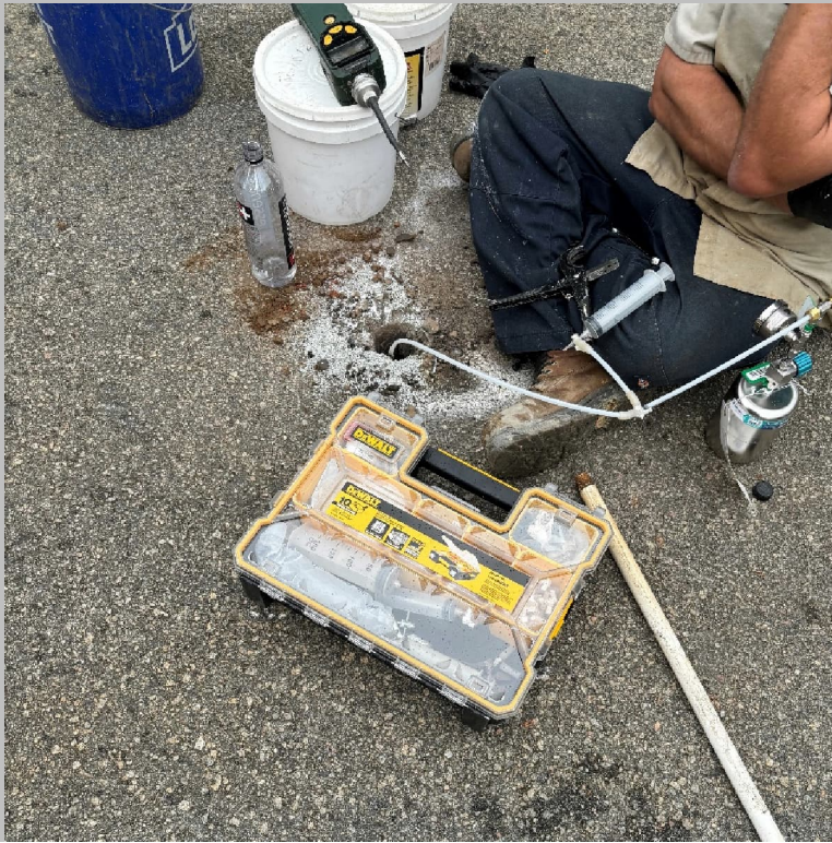
Photograph of soil vapor sampling for SG-2.
